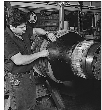
Pulling back cover, tire cord reinforcement and tube prior to building the flanges on an eccentric reducer.
