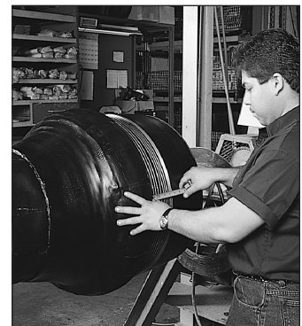
Checking steel wire reinforcement spacing. This guarantees consistently high safety factors.
